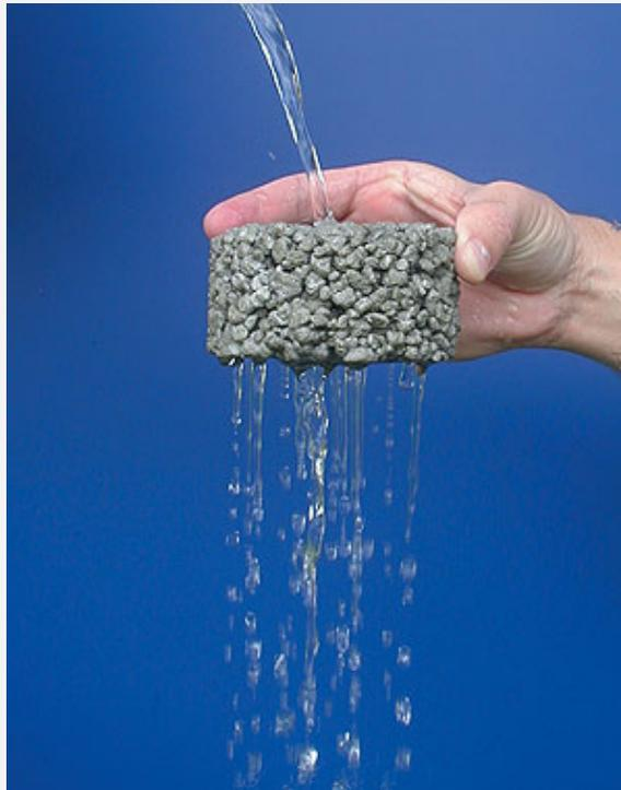
The high flow rate of water through a pervious concrete pavement allows rainfall to be captured and to percolate into the ground, reducing stormwater runoff, recharging groundwater, supporting sustainable construction, providing a solution for construction that is sensitive to environmental concerns, and helping owners comply with EPA stormwater regulations.
